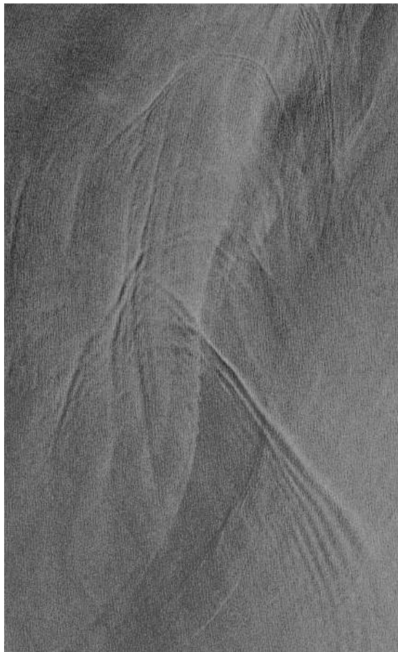
Figure 2. (Right) ERS-2 (C-band, VV) SAR images off Mozambique acquired on 7 January 2002 at 0739 UTC (orbit 35116, frames 4095, 4113, 4131). The image shows the signature of internal waves propagating to the northeast along with current signatures. Imaged area is 100 km x 300 km. ©ESA 2002. (Below) An enlargement showing the internal wave signature. Imaged area roughly 43 km x 70 km. [Image José da Silva Instituto de Oceanografia, Lisbon, Portugal]
