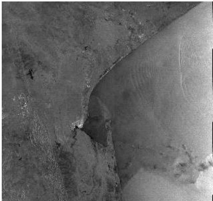
Figure 4 (Right) ENVISAT Wide Swath ASAR (C-band, VV) browse image of the Bay of Maputo acquired on 6 March 2003 at 0717 UTC (orbit 5299, frame 4140). The image shows two internal waves propagating shoreward. Imaged area is approximately 260 km x 260 km. ©ESA 2003. (Below) An enlargement showing the eastern most packet. Imaged area is approximately 56 km x 40 km. [Image courtesy of José da Silva Instituto de Oceanografia, Lisbon, Portugal]
