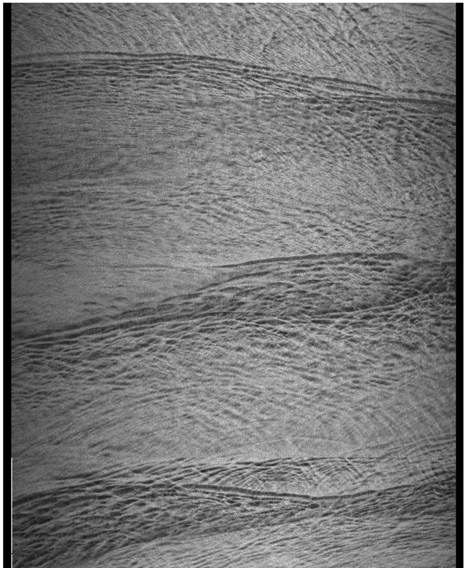
Figure 9. (Left) SIR-C SAR image over the continental shelf off Hong Kong acquired on 20 April 1994 at 0331 UTC (Seg. 9-11). The image shows a very large number of internal wave signatures inside the 200-m isobath (near image bottom). Imaged area is 18 km x 250 km. (Above) An enlargement highlighting the area around the 100 meter isobath (near image center). Imaged area is 18 km x 60 km.
