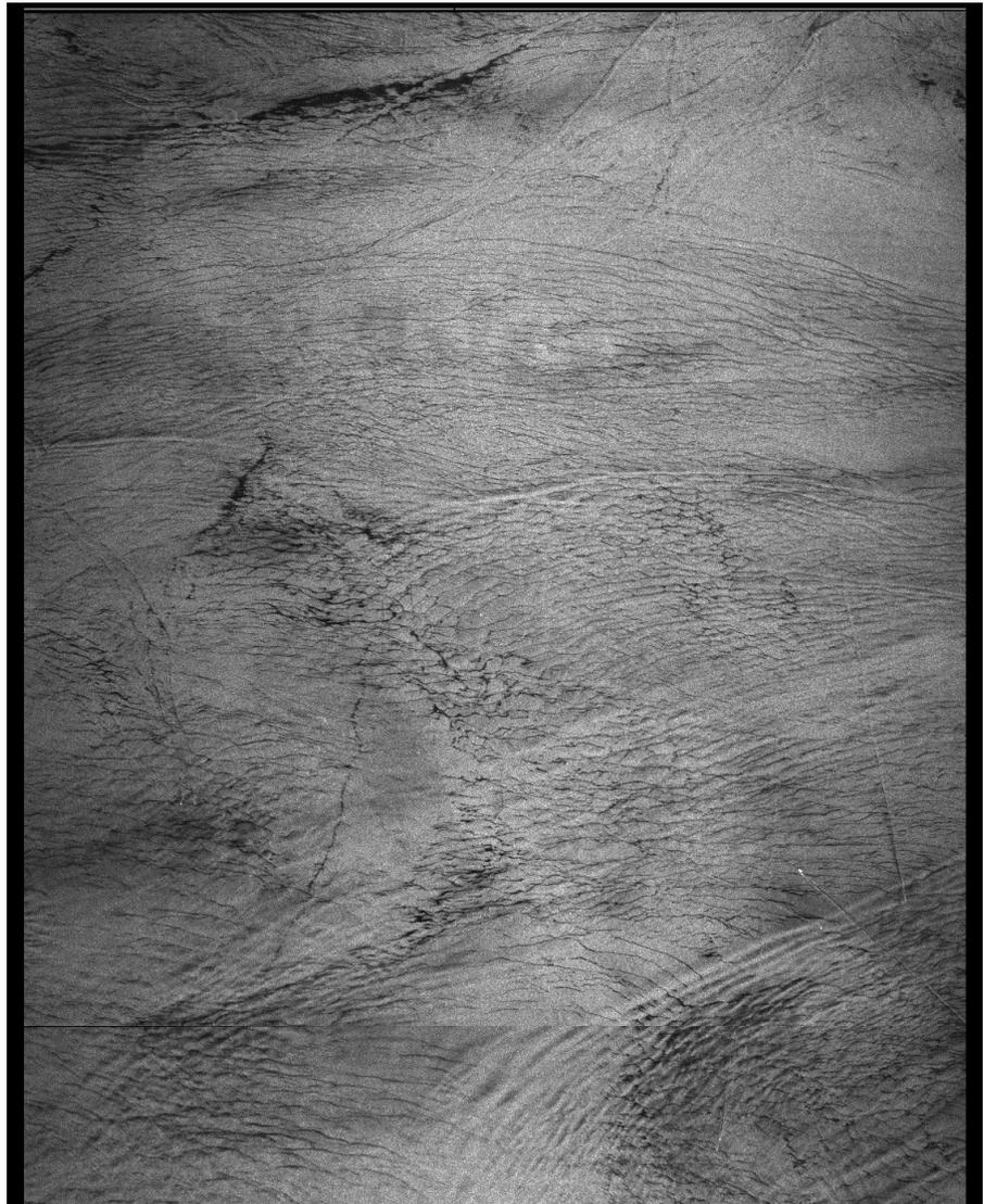
Figure 8. (Left) SIR-C SAR image over the continental shelf off Hong Kong acquired on 20 April 1994 at 0331 UTC (Seg. 9-11). The image shows a very large number of internal wave signatures inside the 200-m isobath (near image bottom). Imaged area is 18 km x 250 km. (Above) An enlargement of the top 60-km section highlighting the large number of wave and their complex interactions.
