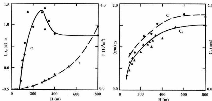
Figure 2. Environmental parameters  $\alpha$  and  $\gamma$  as a function of depth derived from ASIAEX CTD cast data. (See Background and Theory Section 5.1.2). The nonlinear parameter  $\alpha$  crosses zero at depth of 100 m and peaks at approximately 300 m. The difference between  $C$  and  $C_0$  is caused by nonlinear effects.
