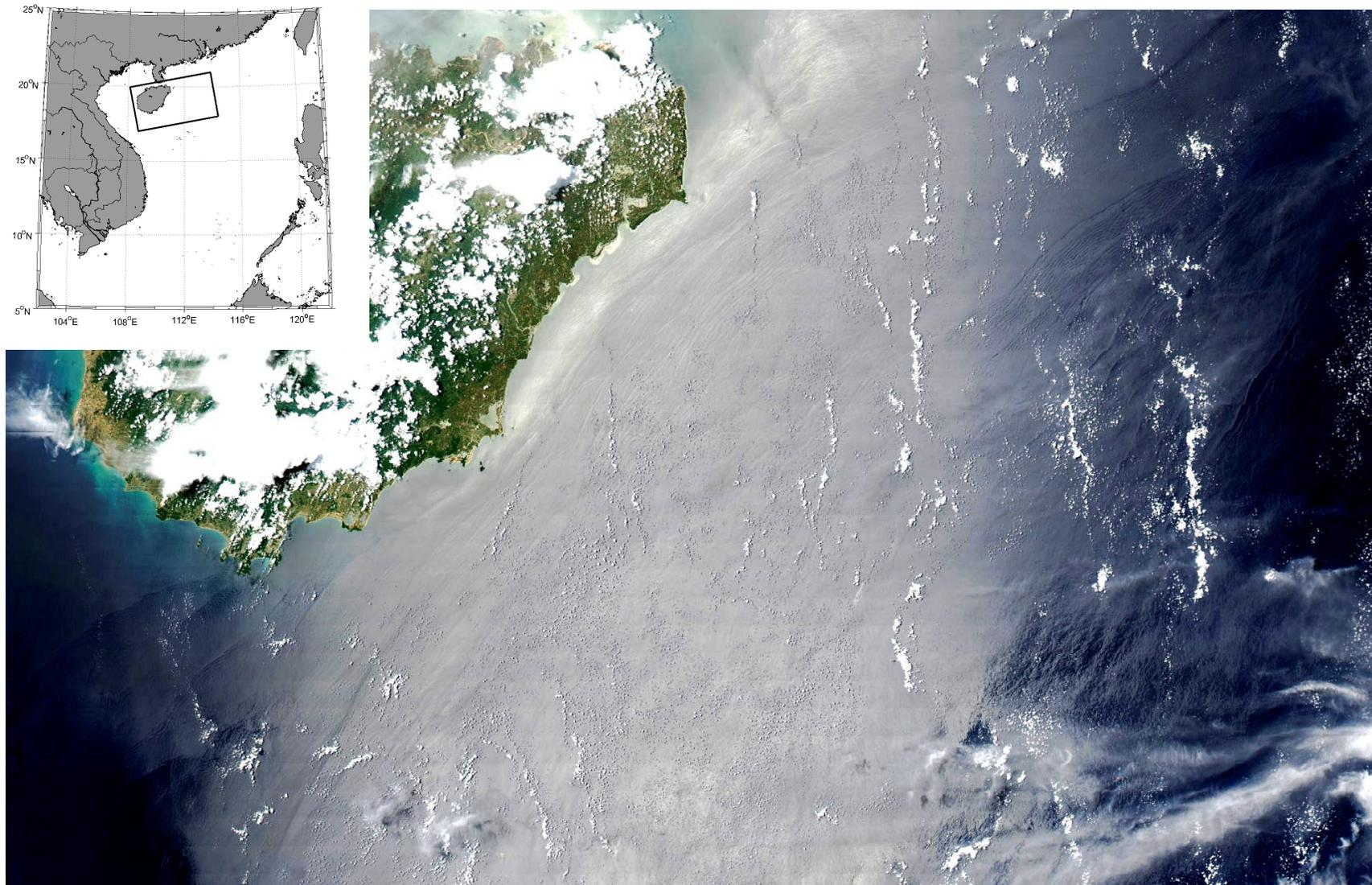
Figure 11. MODIS (Bands 1,3,4) 250-m resolution visible image over Hainan Island in the South China Sea acquired on 9 July 2003 at 0545 UTC. The image shows internal wave packets east (top right) and south (bottom left) of Hainan Island propagating to the northwest. Less well organized surface signatures are visible immediately east of the island. Imaged area is approximately 500 km x 325 km.
