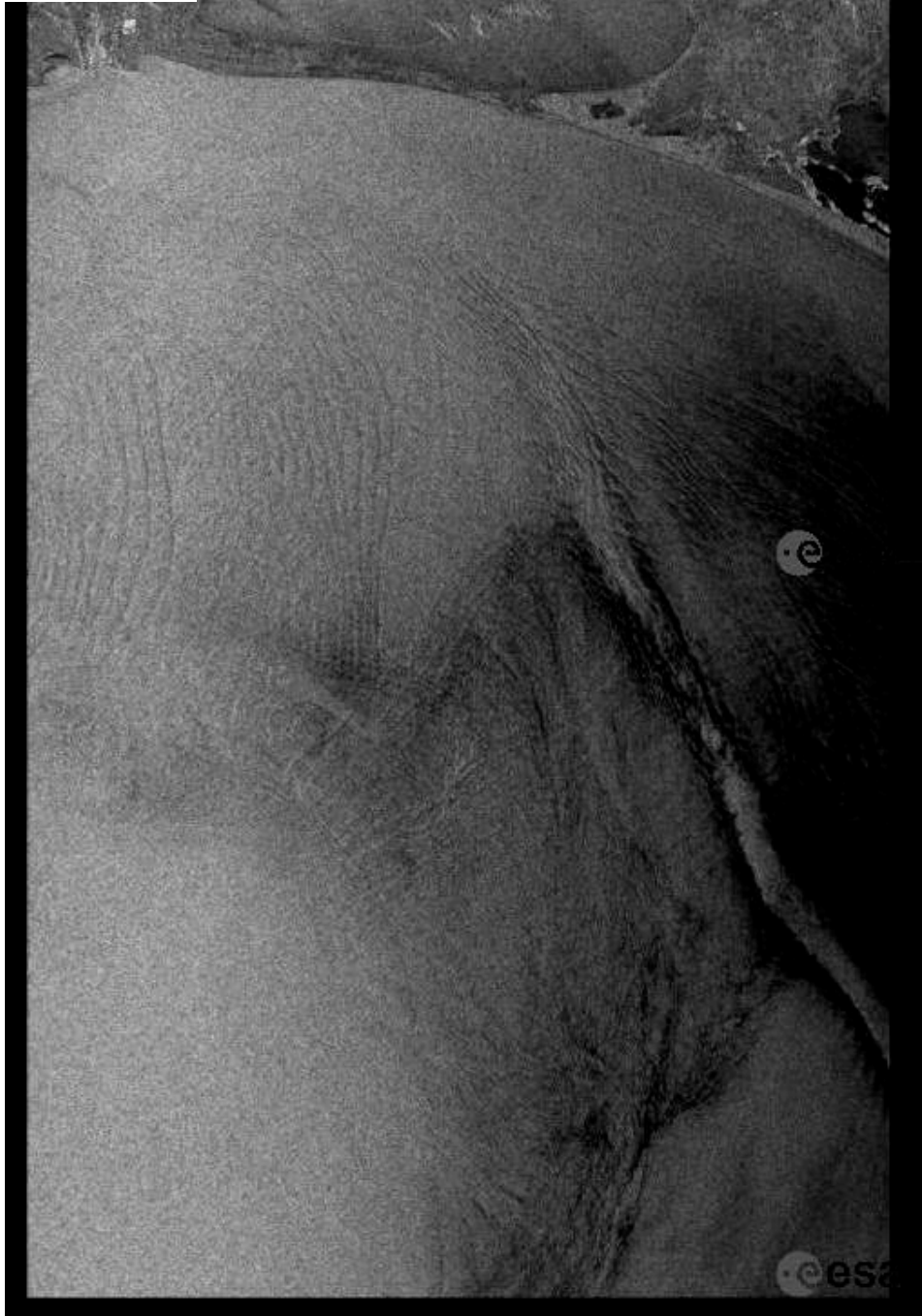
Figure 2. ERS-2 (C-band, VV) SAR survey image of the Gulf of Tehuantepec acquired on 30 March 1996 at 0450 UTC (orbit 4926, frames 297 and 315). The image shows the signature of several internal wave packets propagating shoreward. Imaged area is 100 km x 200 km. ©ESA 1996.
